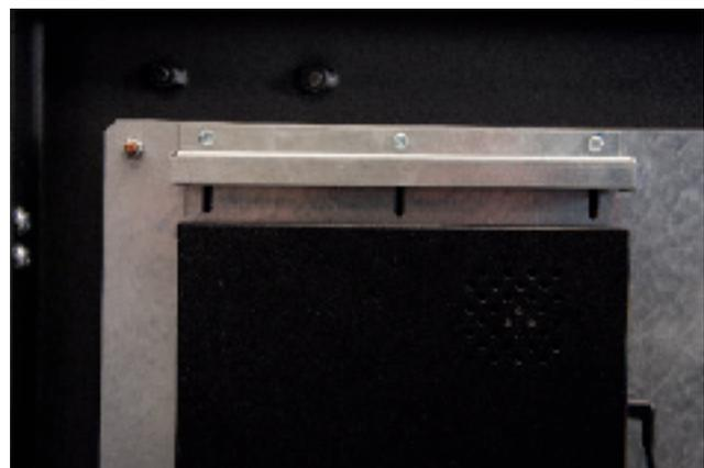
If the S-Box is operated separately, all cables must be routed through the brush strip to the inside. The S-Box power supply unit can be detached from the mounting plate (attached with Velcro).
